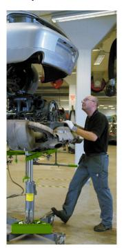
blies, rear axles, gearboxes, fuel tanks, exhaust systems and much more. With its lifting capacity of almost 550 kg, the HTJ1200 universal handling system comes with enough power for all kinds of jobs
